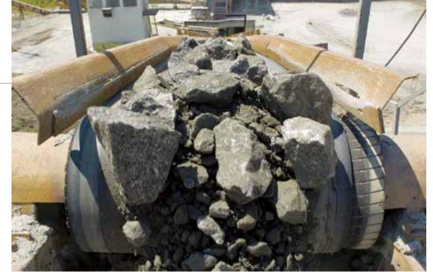
replace the steel cord conveyor belt with a PN (polyester-nylon) textile conveyor belt one supplied by Mercurio" said Clermont, referring to a product that can endure severe application conditions.
