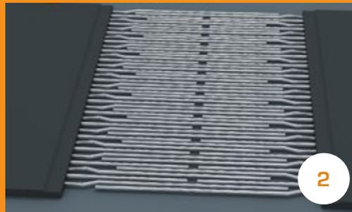
The cement is then applied to the steel cables and also to the Chamfer region. After drying, start assembling the splice in the following order: insert the silicone paper, the lower covering rubber and a core rubber blanket. Then, the steel cables are transposed, which must be started from the center to the edges of the belt, ensuring their centralization and alignment. The empty space between the cables must be filled with the core rubber, the so-called
