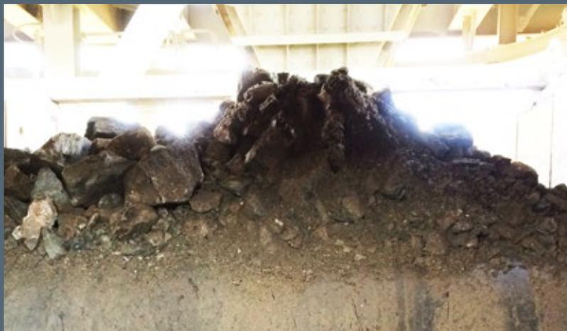
**BY CHANGING THE BELT COVER FROM EA TO MERCORIP AND INCLUDING AN ARAMID RIP PROOF MESH, THE MERCURIO TECHNICAL TEAM HAS DOUBLED THE BELT’S SERVICE LIFE, PROVIDING GREATER SAVINGS AND PRODUCTIVITY TO THE CUSTOMER.**
