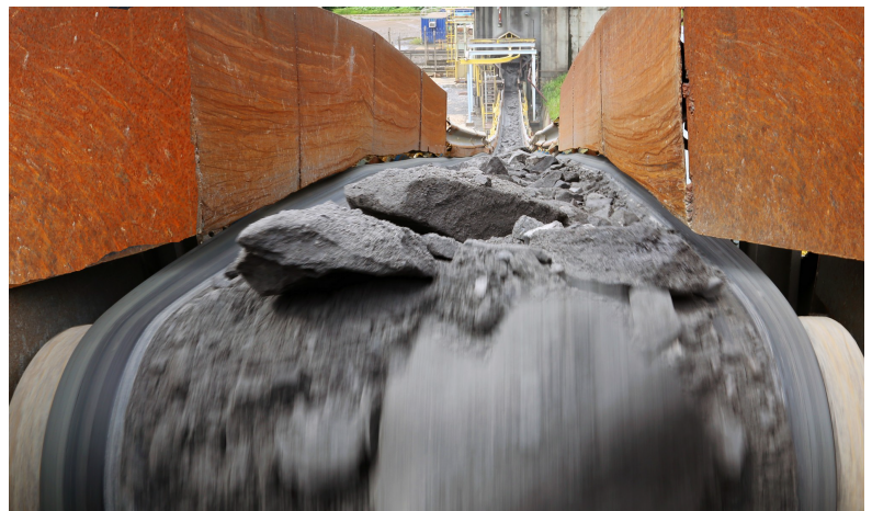
MercoRip conveyor belt operating in a severe impact and abrasion application.
